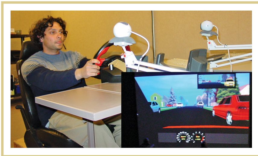
Figure 1. A study participant being monitored in the STISIM driving simulator. The simulator runs on a single PC and projects the image of the roadway onto a white wall in the lab.
